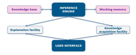
Figure 3. Architecture of an expert system (own elaboration).
