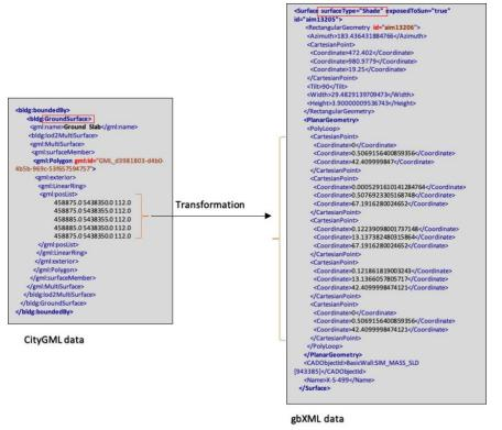
Figure 8: The gbXML and CityGML XML files
