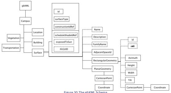
Figure 30: The gbXML Schema
