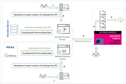
Figure 5: Software architecture of the two services implemented according to the first methodology
