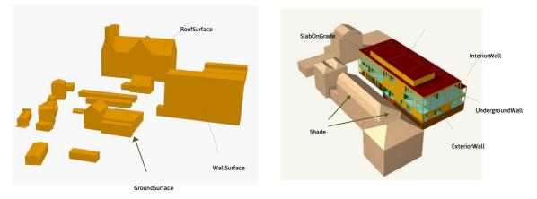
Figure 7: gbXML data and its surfaces VS. CityGML data LOD2 and its surfaces
