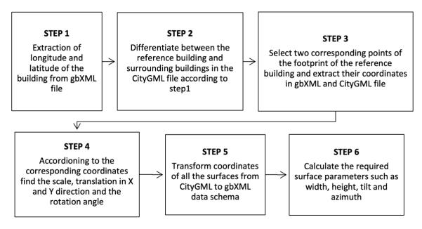
Figure 10: Workflow of transforming CityGML surface to gbXML surface
