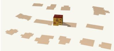
Figure 20: Integration of footprints of the surrounding buildings with gbXML data
