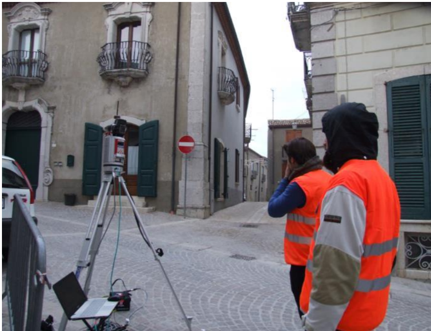
Figure 34 – Laser scanning of Frigento Demo Case with the use of RIEGLE
