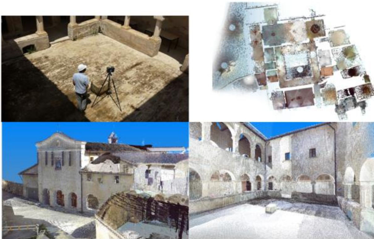
Figure 43 – JRC 3D RECONSTRUCTOR results from FARO survey. Convento Sant’Angelo d’Ocre, L’Aquila (IT)
