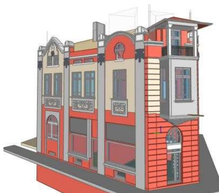
Figure 12: BIM model with final renovation scenario for demonstration project #7 Historic residential building in Varna
