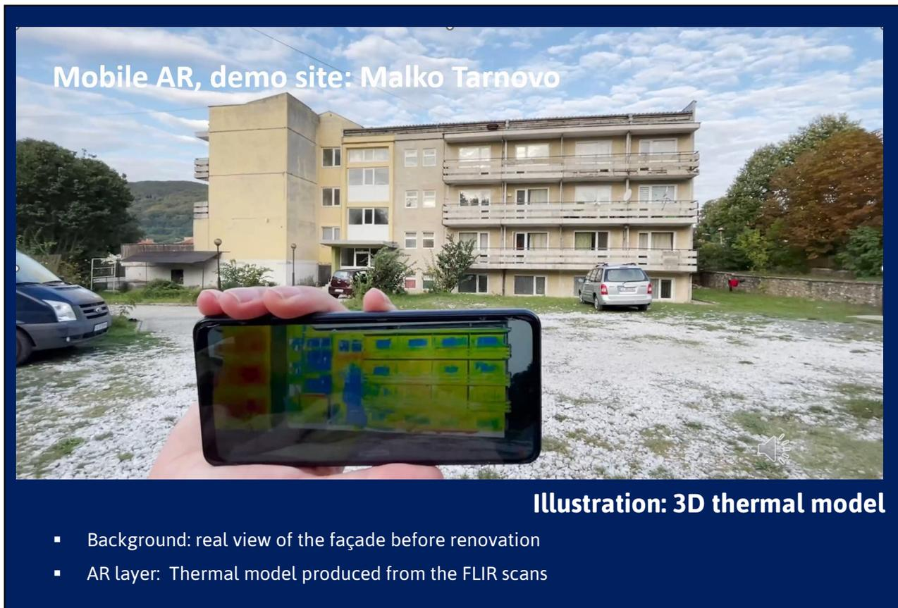
Figure 20: On-site demonstration of the 3D thermal model of demo site Malko Tarnovo, 2022
