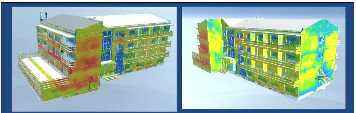
Figure 79: 3D thermal images based on 2D thermal scans
