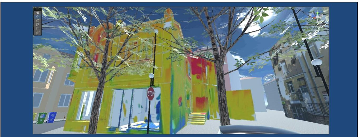
Figure 71: Thermal 3D model based on 2D geo-thermal scans, view from the smaller street (Bdin str.)
