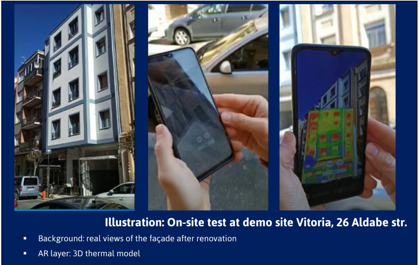
Figure 39: On-site test mobile demo site Vitoria, 26 Aldabe str.
