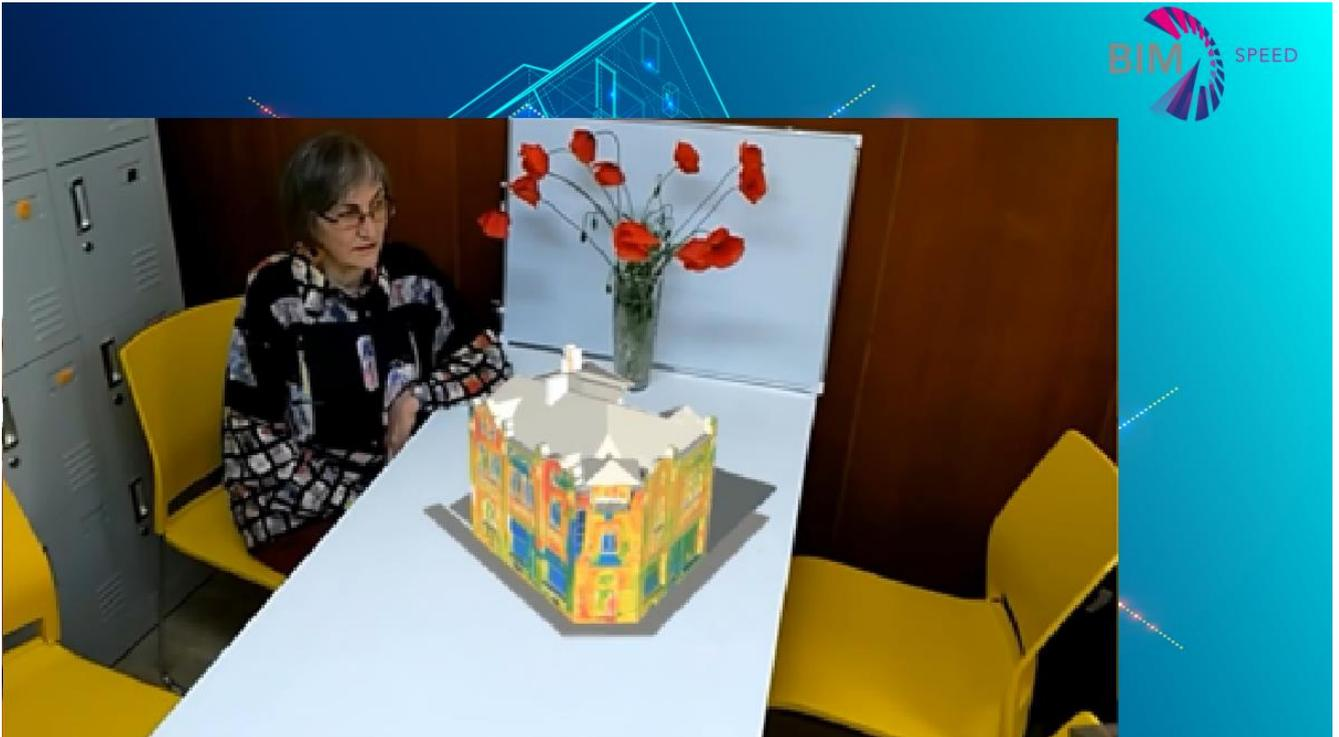
Figure 55: Small-scale hologram of a 3D thermal model
