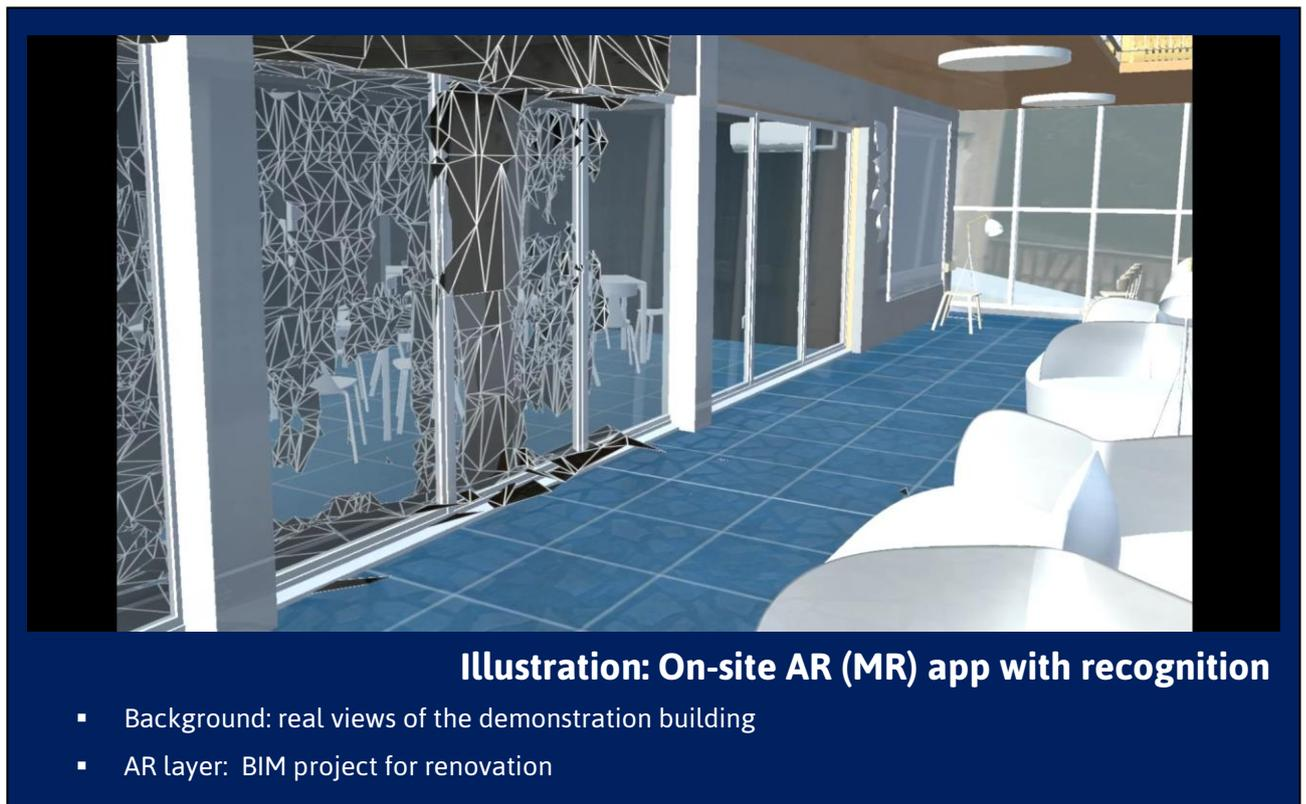
Figure 60: Process of overlapping the real building with the holographic BIM model for renovation
