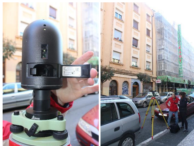
Figure 11: 3D laser scanning (Source: BIM-SPEED)
