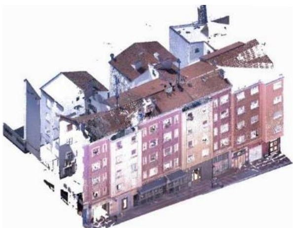
Figure 13: Point cloud model (Source: BIM-SPEED)
