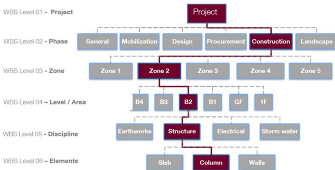
Figure 24 – Project Breakdown Structure (example)
