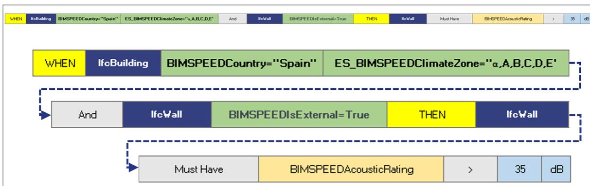
Figure 18 - Example of Transition of Design Rule to checkable format
