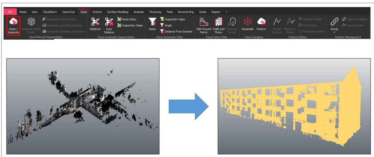
Figure 48 - Purging the point cloud
