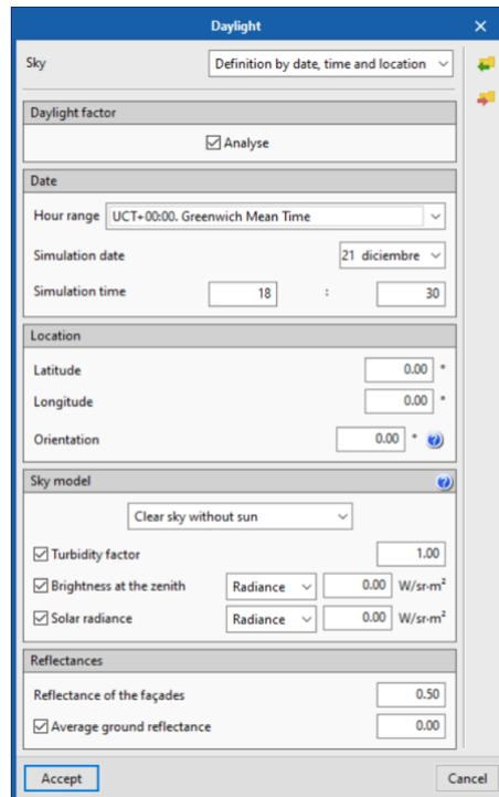
Figure 27: Daylight definition in CYPELUX
