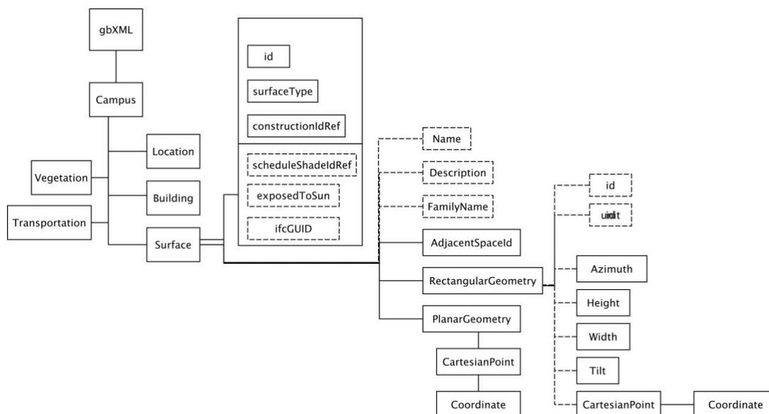
Figure 30: The gbXML Schema
