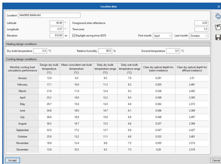
Figure 24: ASHRAE Weather Data Viewer location data – 'Flexible' panel
