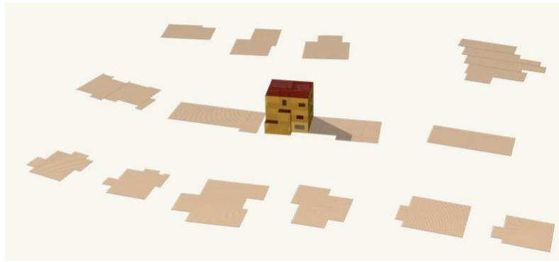
Figure 20: Integration of footprints of the surrounding buildings with gbXML data
