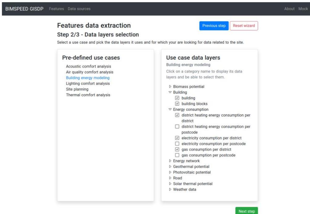
Figure 18: Required surrounding data for building energy modelling
