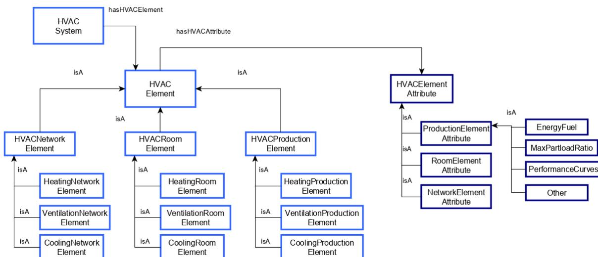
Figure 27. HVACSystem and Element classes
