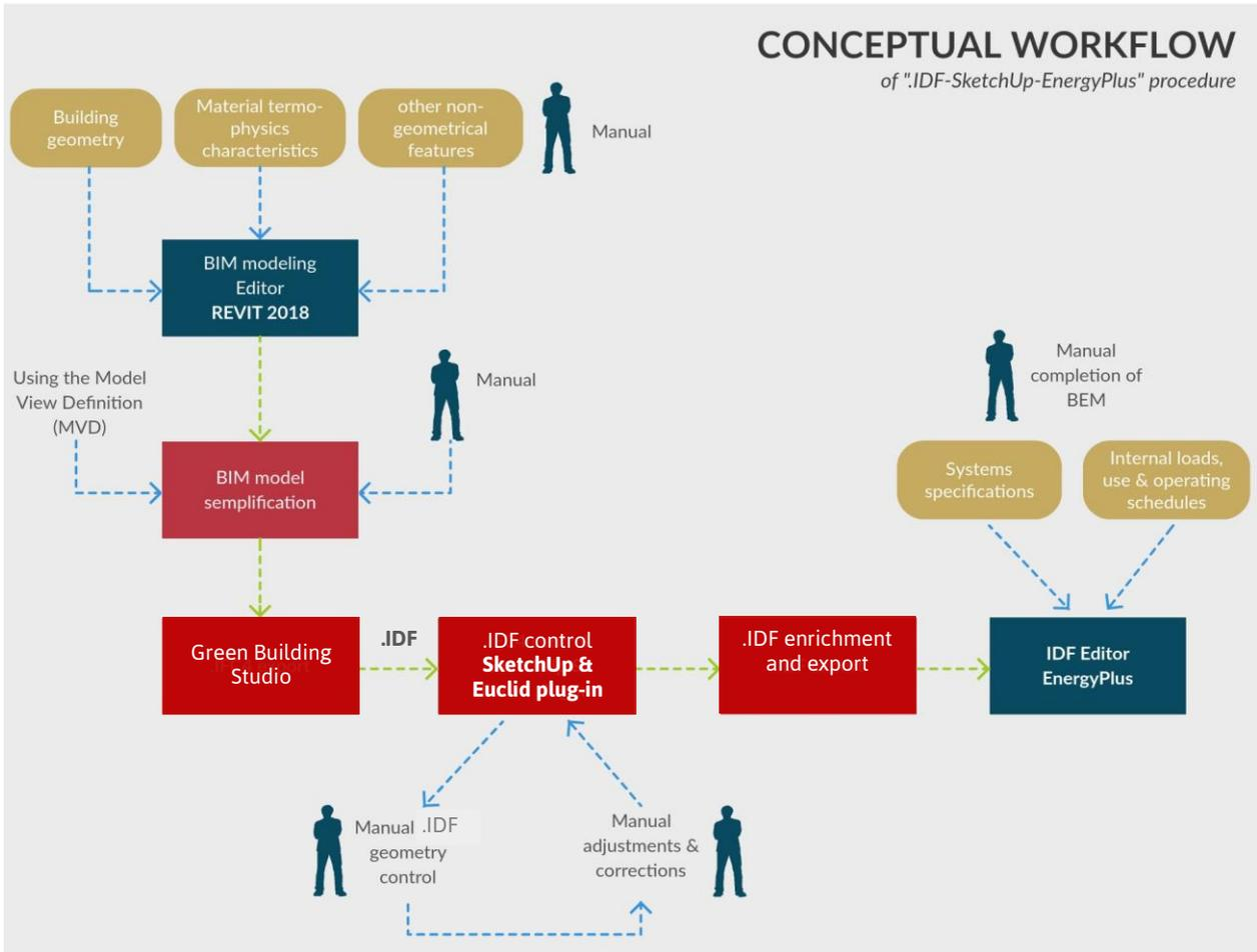
Figure 22.Revit – SketchUp (with Euclid plug-in) – EnergyPlus” BIM-to-BEM procedure (BIM-SPEED 2019b)
