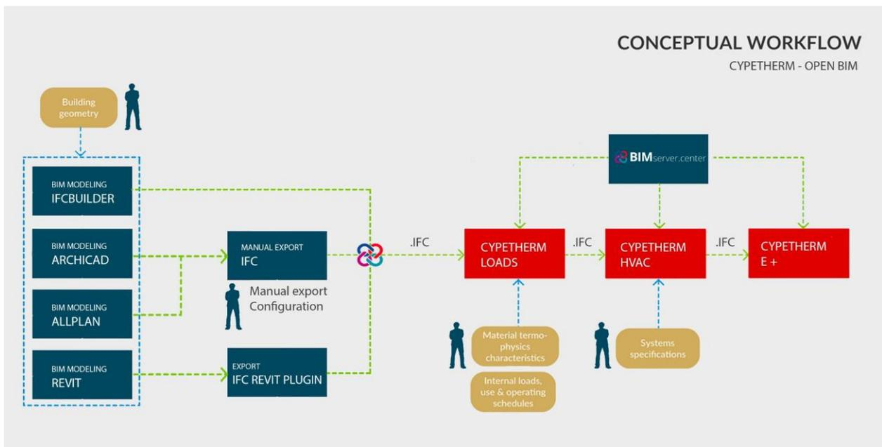
Figure 21. “IFC-CYPETHERM Suite” conceptual workflow of the procedure (BIM-SPEED 2019b)
